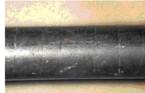
Ammonia-induced cracking of the 5 Cr-0.5 Mo alloy
