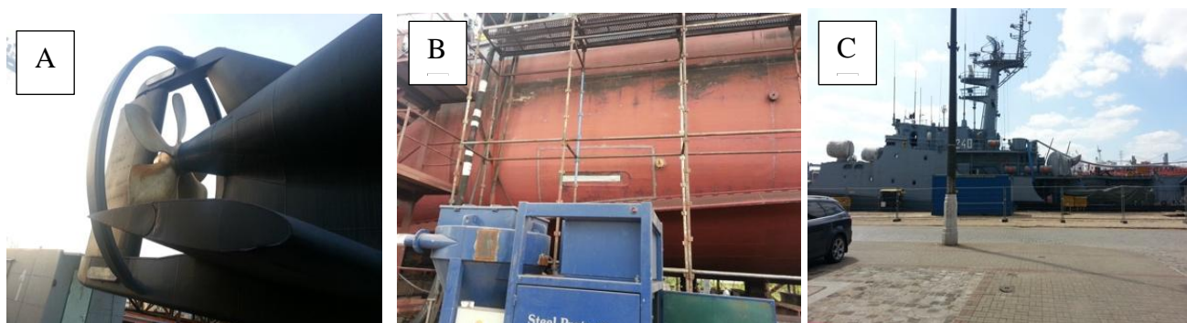
Photo. 4.14. (A) Submarine propeller, (B) Ship in dry dock; on the ship hull, there is a visible screen including the anode, (C) Warship at the quay during polarization tests.
