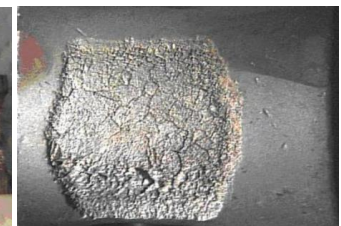
Selective dissolution of nickel from Monel. Presence of oxygen in hot HF
