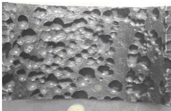
Metal dusting. Furnace pipe made of 304 steel
