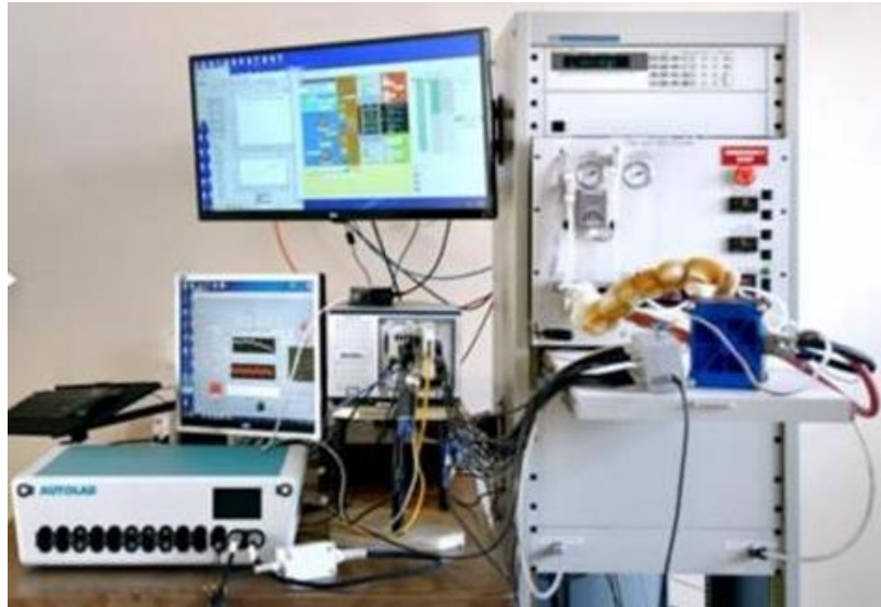
Photo. 4.11B. Digital Dynamic Electrochemical Impedance Spectroscopy measurement system based on National Instruments measurement cards coupled to a hydrogen fuel cell test bench.
